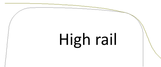
Severe gauge-corner contact
